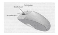
**Mouse**: The device that controls the movement of the pointer displayed on the screen. You use the mouse pointer to select and open items on the computer.
