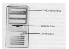
**Disk drives**: Devices that read data from and write data to a disk. A DVD drive reads both CDs and DVDs. A DVD
